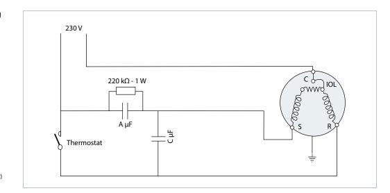
IOL Motor protector A & C Run capacitors C Common
