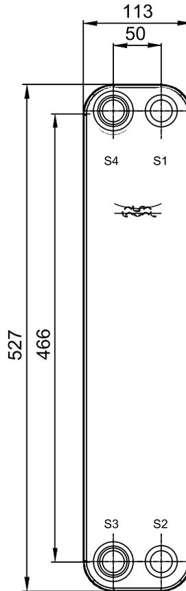
Frameplate is depressed 2.1 mm at connections S3 and S4 if holed.
